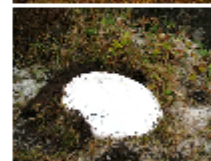
Figure 3: The litter trap consisted of a plastic bucket dug into the ground so the brims were parallel to the ground.
