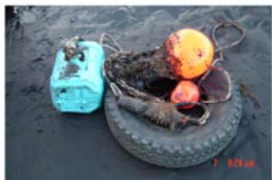
Figure 3. In the lagoon and in the sea the receivers were fastened to a rope attached to a float and a sinker (the tire is not part of the equipment).
